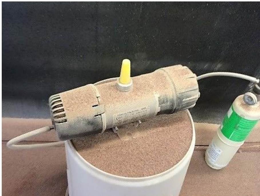
Image 3: Successful gas test for detector during grit blasting assessment
