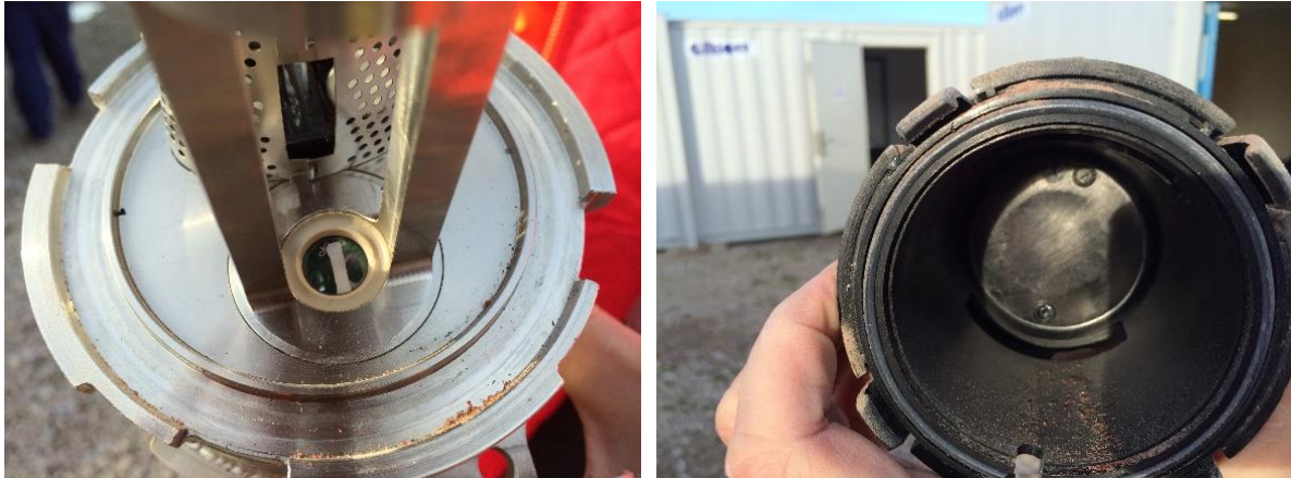
Image 4 & 5: Clean optics on GasSecure GS01 gas detector after grit blasting tests
