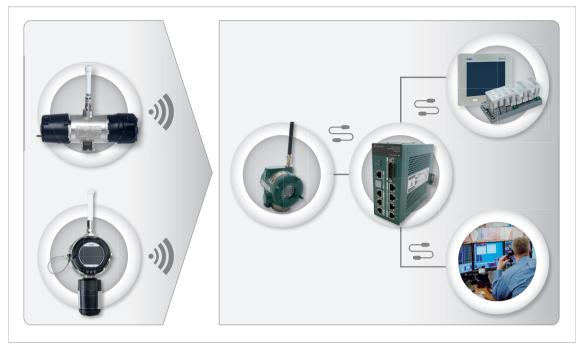
The wireless transmitter send their detection signal to the access point. From there, the signal is transferred to the gateway, which feeds the control unit directly via Modbus or with the PROFINET® protocol.
