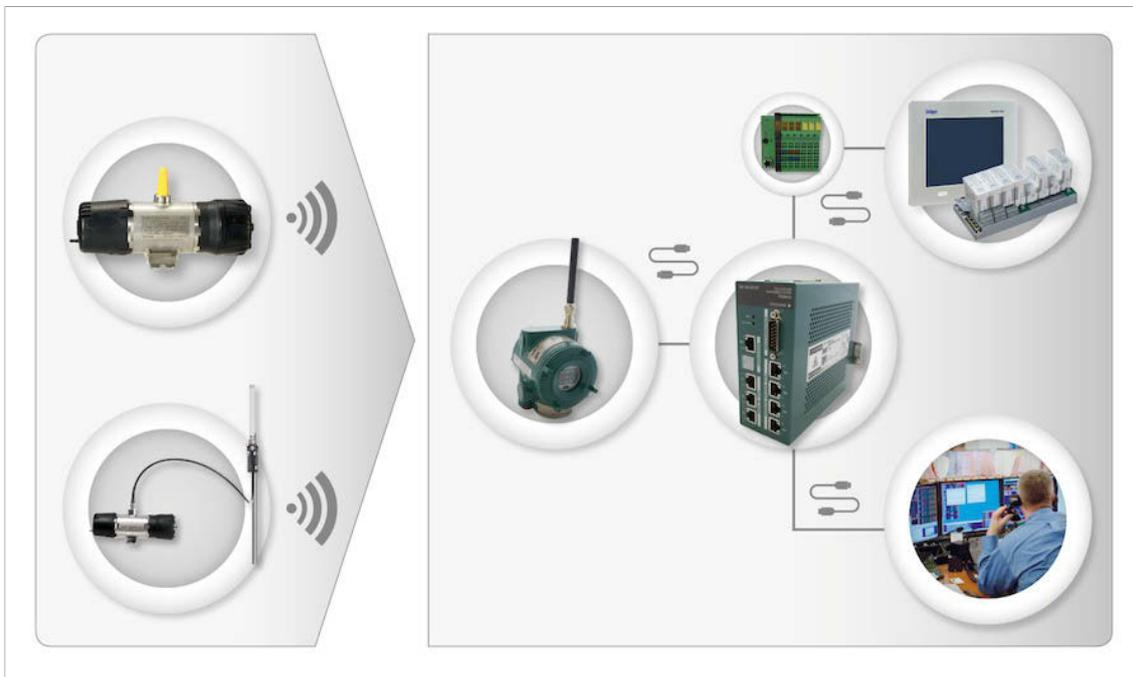
The GS01 transmits its detection signal wirelessly to the access point. From there, the signal is transferred to the gateway. This feeds the control unit directly via Modbus or with the PROFINET® protocol. For analogue analyser units, a D/A converter can alternatively be used.
